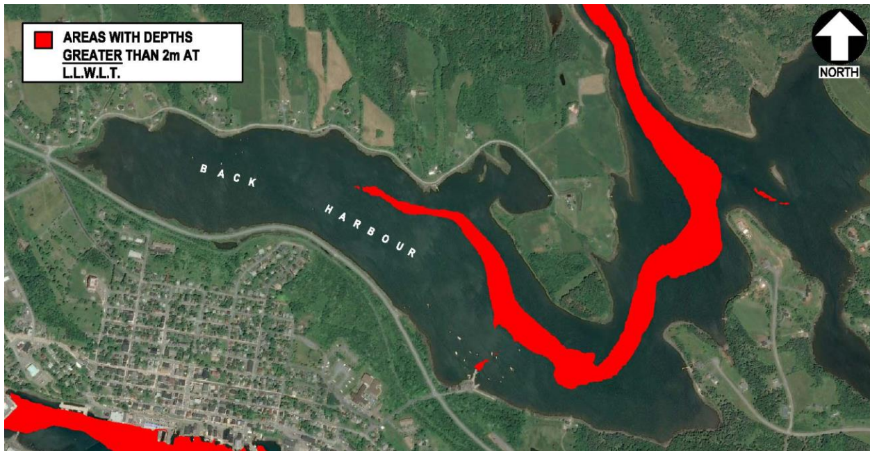
Figure 2: Option 1- Red shaded areas represent areas with depths of water sufficient to terminate an outfall at as per Atlantic Canada recommendations.
