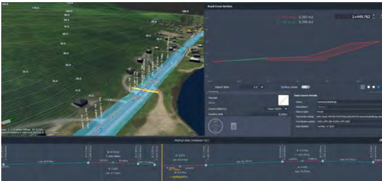
Figure 5-2: InfraWorks Design Process
