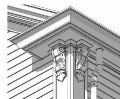
PROPOSED SOLUTION: CONTINUOUS FASCIA FROM EAVE RETURN ACROSS FRONT AND BACK OF THE HOUSE THAT WILL CONCEAL THE GUTTER.
