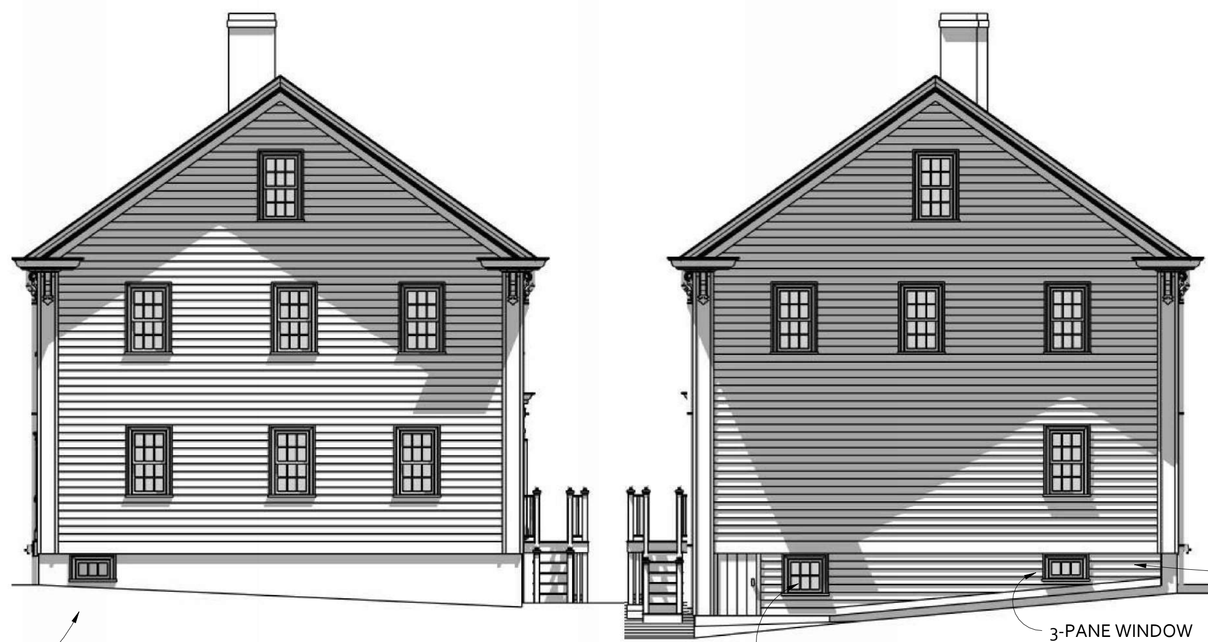
PROPOSED SOLUTION: CONTINUOUS FASCIA FROM EAVE RETURN ACROSS FRONT AND BACK OF THE HOUSE THAT WILL CONCEAL THE GUTTER.
