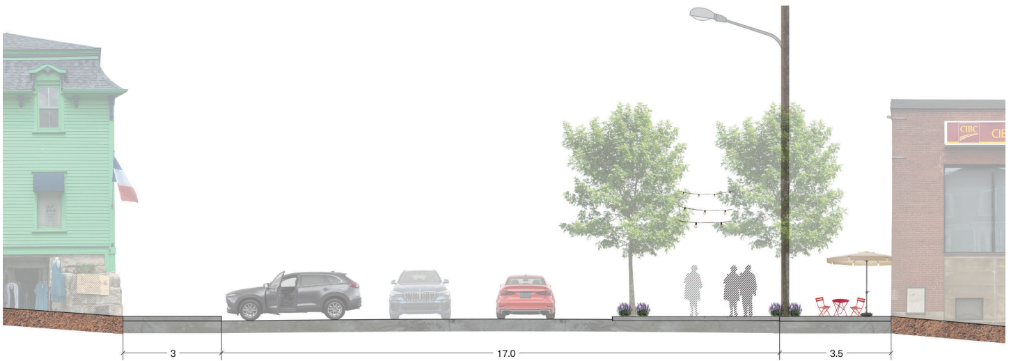
Figure 8.4 King Street Widened Sidewalk / Linear Park
